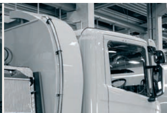
Additional water tank
