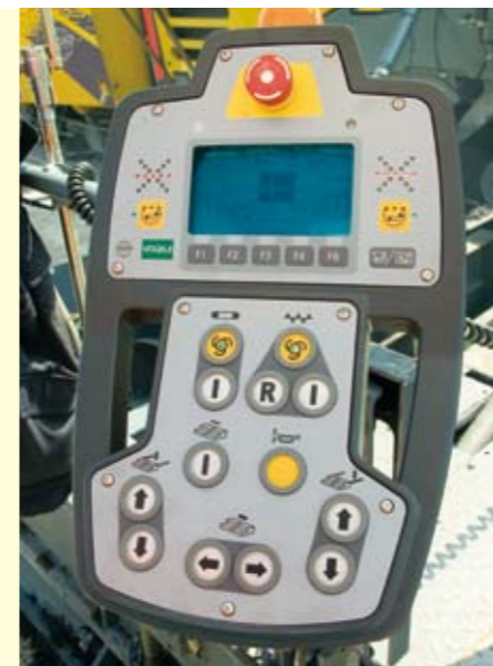
Clearly arranged: the NAVITRONIC® Plus operating console for the screeman.
