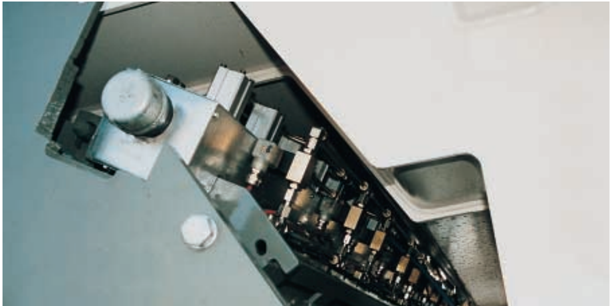
The spraybar directly above the milling and mixing chamber of the Wirtgen Recycler WR 2500 consists of 16 nozzles with expansion chambers in which the hot bitumen is foamed and then evenly sprayed as foamed bitumen over the complete working width.
