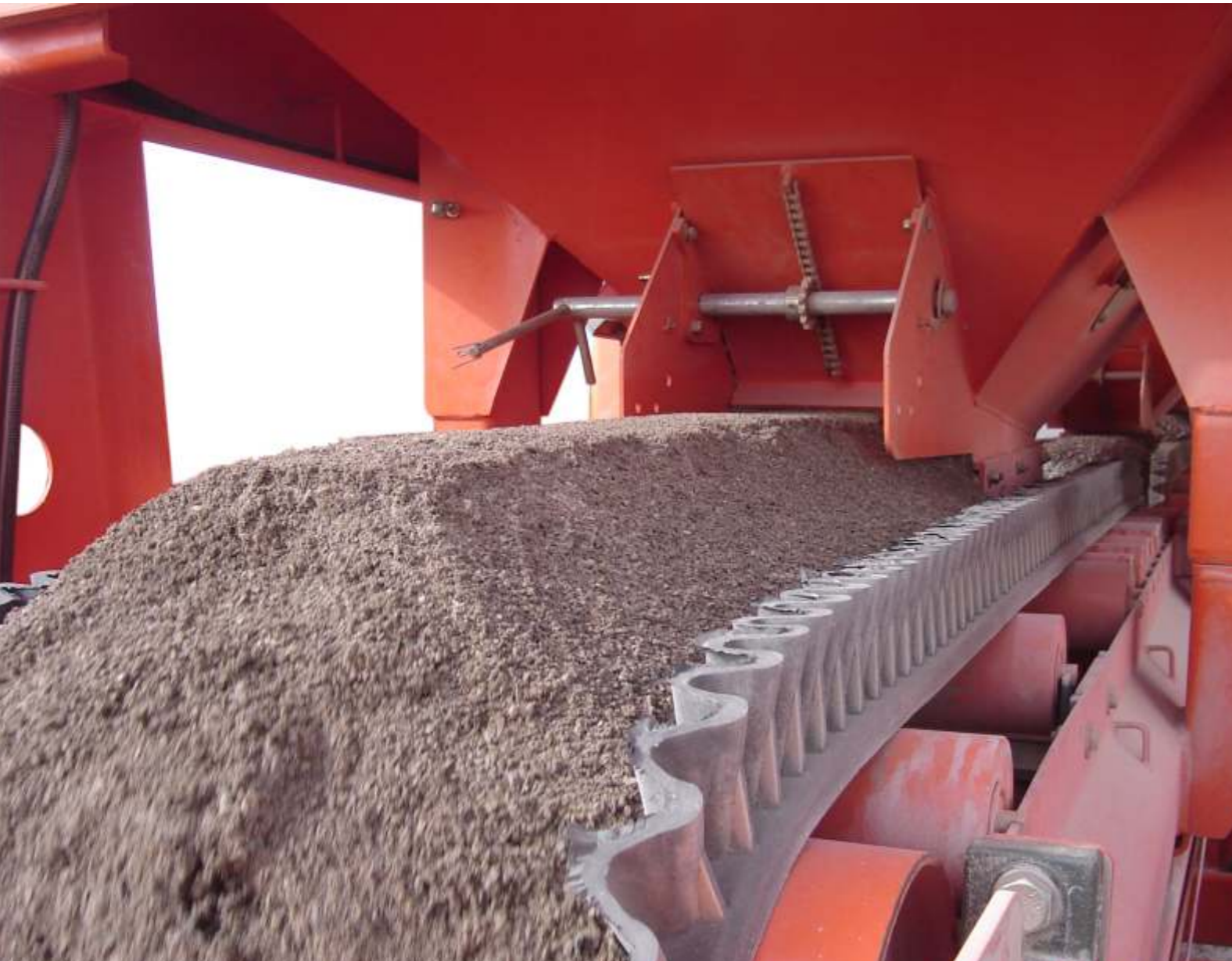
Dosing belts with vulcanized side guards
