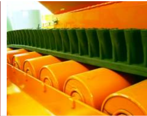
Dosing belts with vulcanized side guards
