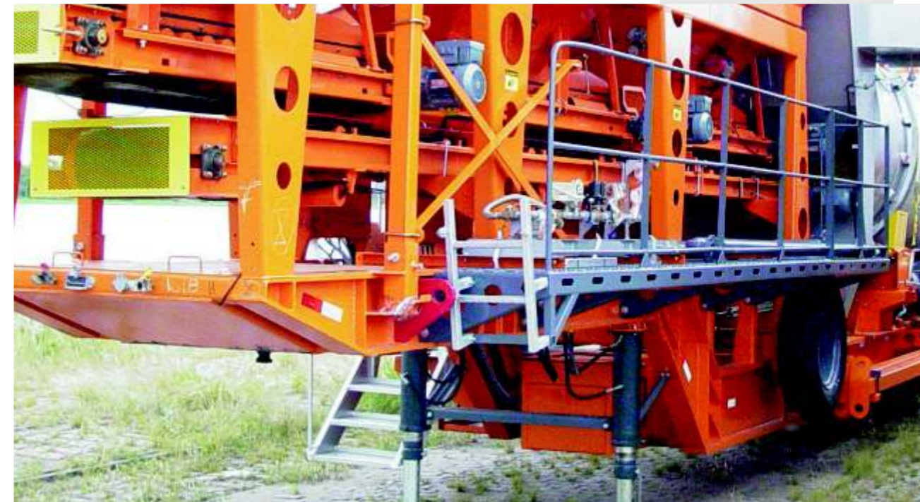
Inspection Platform for the Bins
