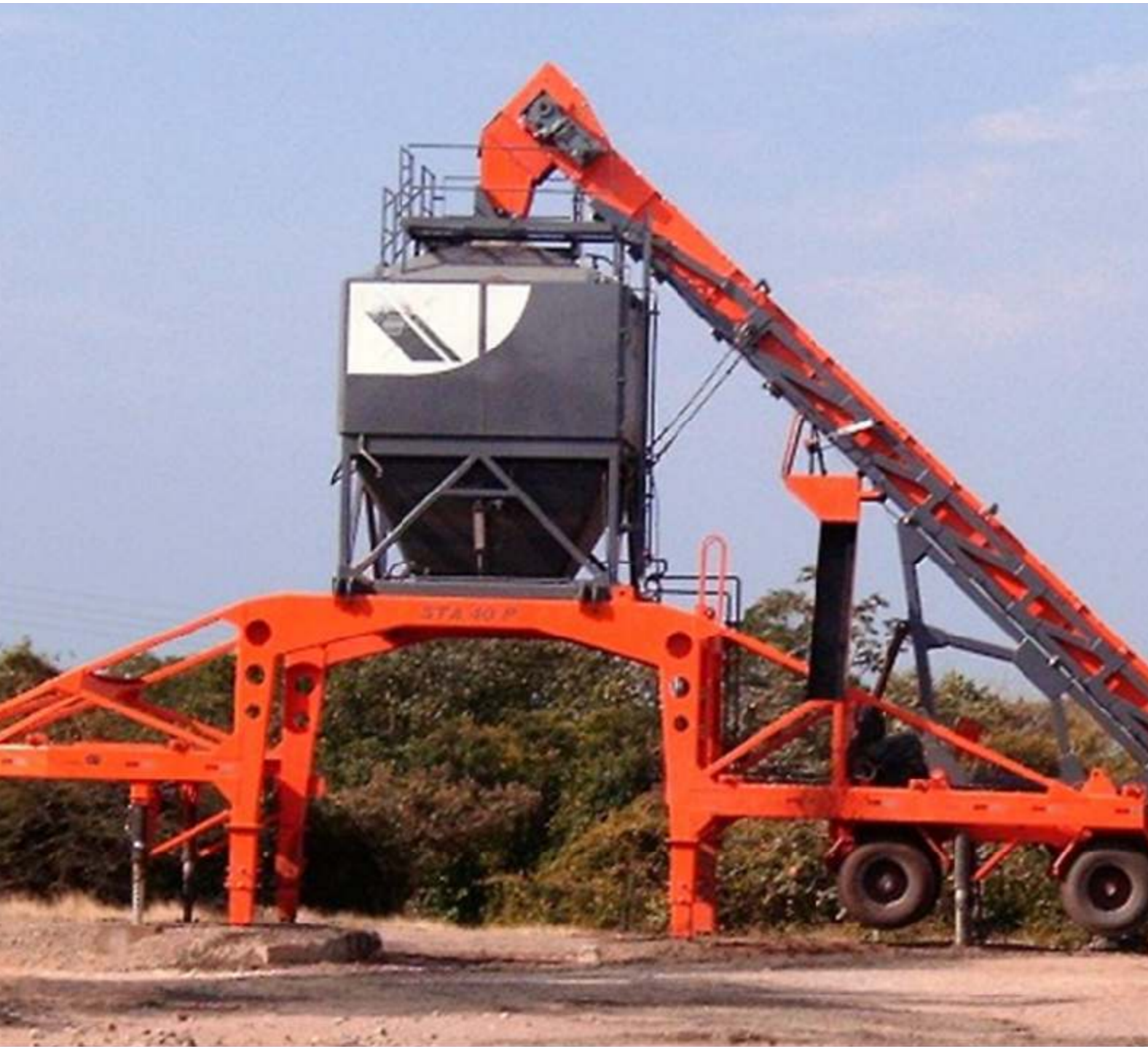
Plant with an Asphalt Storage System
